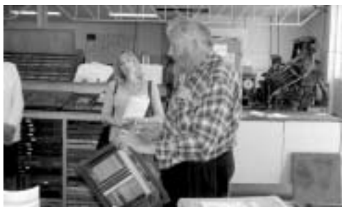
Michael explaining the mysteries of composing. The upper and lower cases are on the left, and the linotype machine on the right.
